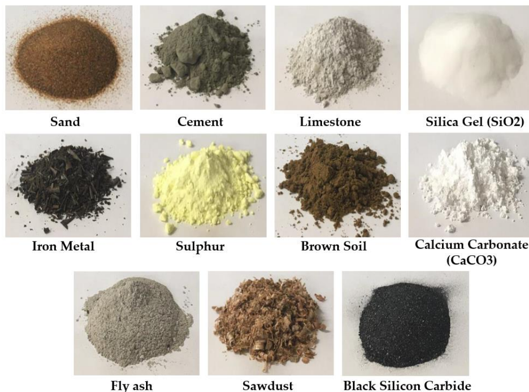
Figure 5. Raw Materials of different categories of dust components [37].
