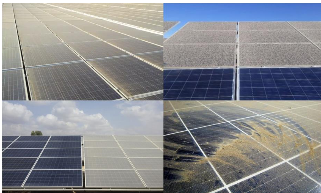
Figure 3. Scenario of natural dust accumulation on solar photovoltaic panels in different locations.
