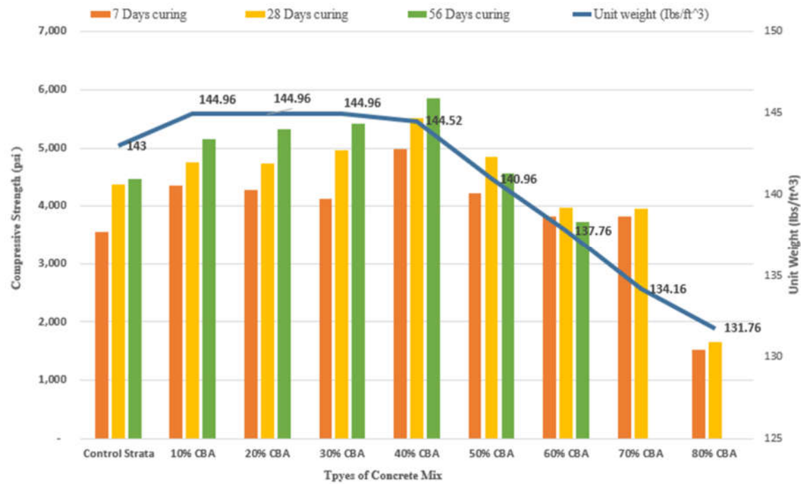
Figure 5. Strata Control and %CBA concrete unit weight vs compressive strength.
