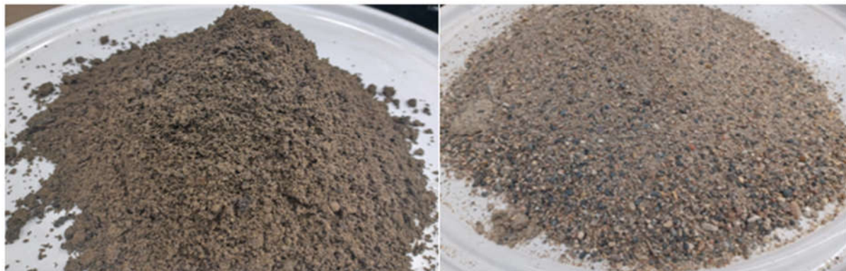
Figure 1. CBA (left) and fine aggregate (right).
