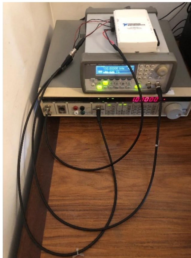
Figure 7. Hardware setup used to experimentally validate the relationship between jitter and estimated sinewave amplitude. Two function generators were used together with a 16-bit data acquisition module from National Instruments, model NI-USB-6218 (seen on top) connected through a USB interface with a personal computer (seen partially on the right). One of the function generators, model DS360 from Stanford Research (bottom) was used to create the sinusoidal stimulus signal. The other function generator, model AG3320A from Agilent (middle), was used to create the clock signal that controlled the sampling instants, and which was modulated by internally generated, normally distributes, phase noise.
