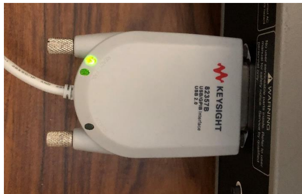
Figure 10. Photograph of the USB/GPIB Interface module from Keysight, model 82357B connected to the Stanford Research DS360 generator to the right. The cable to the left of the image has an USB interface and goes to the personal computer.
