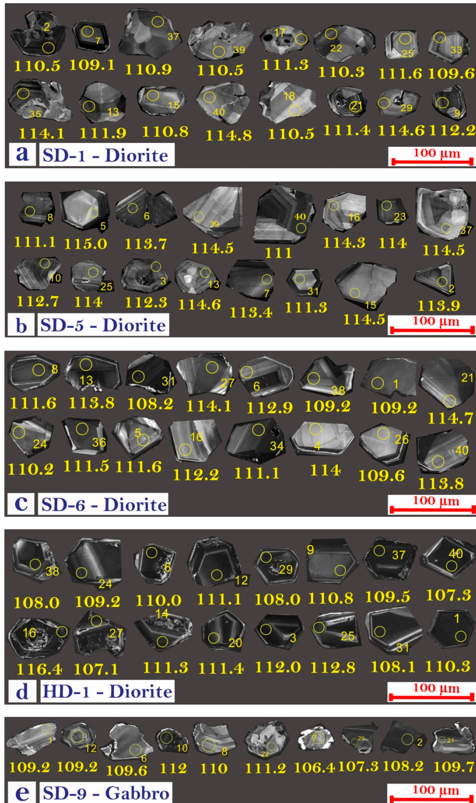
Figure 5. Cathodoluminescence (CL) images of the analyzed zircon grains from the studied samples of Danyore Valley copper-gold prospect, Northern Pakistan. Yellow colored circles show the LA-ICP-MS analysis of the U-Pb dating spot.
