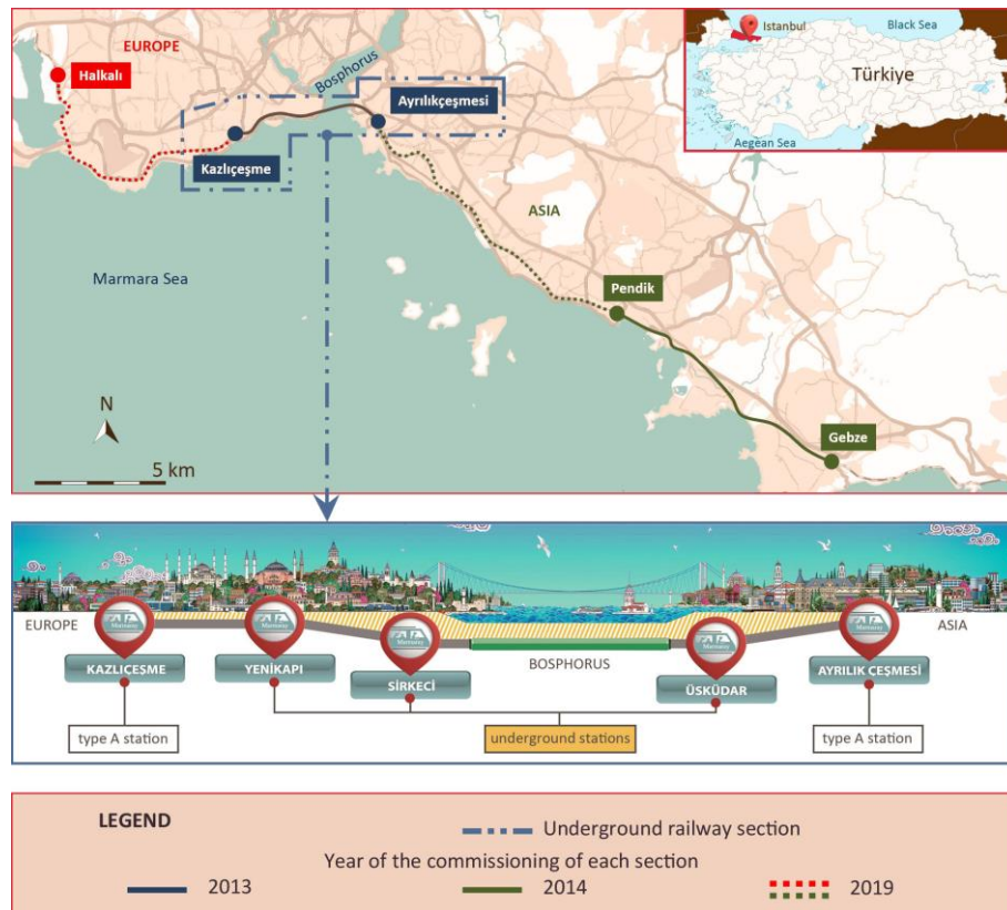
Figure 3. Explanatory maps and sections of the Marmaray railway. Source: Own elaboration based on the contract specifications of BC1 and CR3 (DLH, 2010), Railway Gazette International and “MetroIstanbul 2016”.
