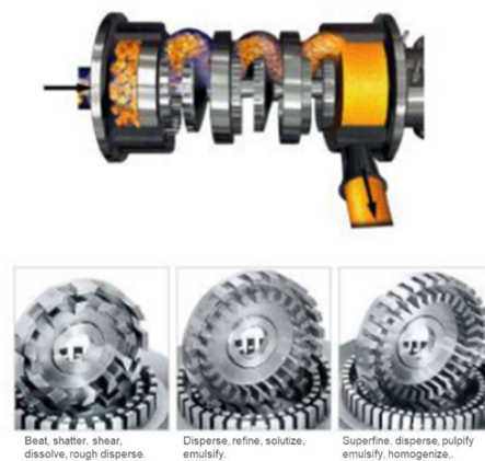
Figure A2. Three-stage rotor-stator tri-emulsifying pump (TRL-L3-60, Wenzhou Rayen Machinery Co., Ltd., China), powered by a 4.0 kW Siemens motor operating at 2900 rpm.
