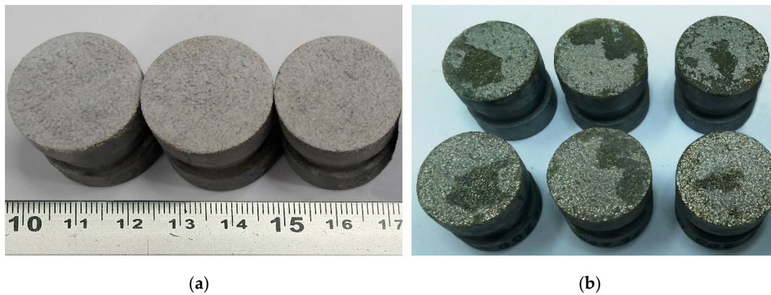
Figure 8. External appearance of samples sprayed with HA coating on Zr sublayer for measuring the adhesion strength for normal peel: (a) before testing; (b) after testing.
