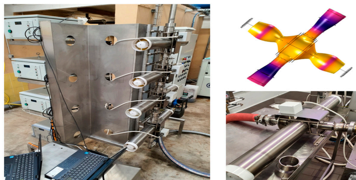
Figure 3. Four ultrasonic units mounted in vertical.
