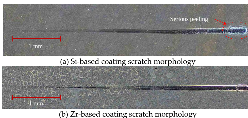
Figure 20. Scratch morphology of Si-based coating and Zr-based coating.
