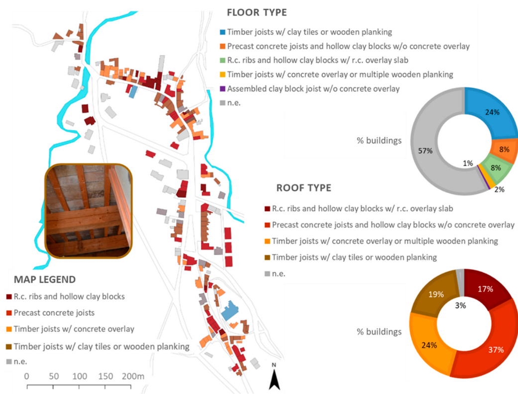
Figure 4. Distribution of roof types in buildings of Pievebovigliana: map with example of traditional solution (timber joist with clay tiles in picture) and diagrams of relative frequency of diaphragm types (floors and roofs).
