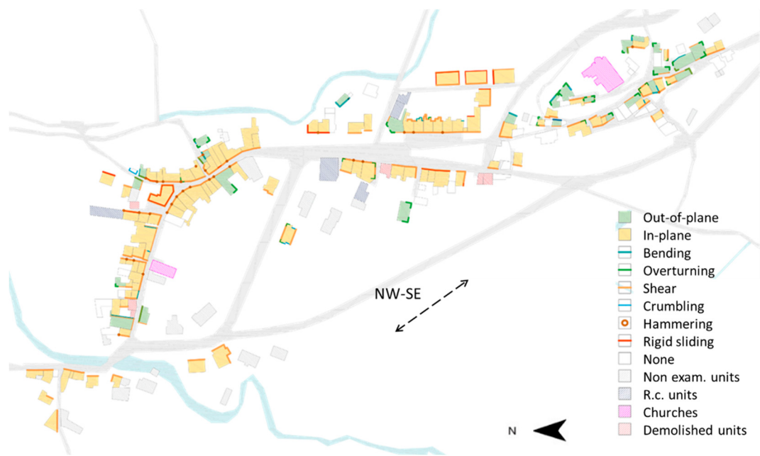
Figure 9. Distribution of main mechanisms activated on building facades in Pievebovigliana according to main orientation of seismic swarm.
