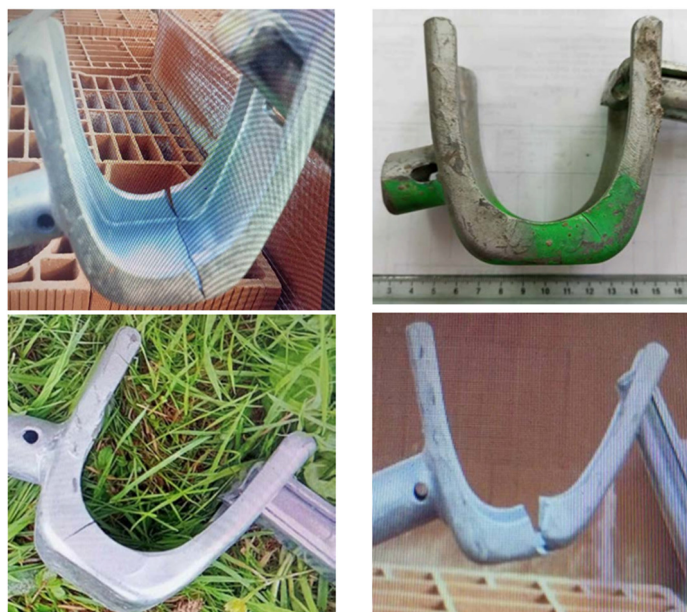
Figure 1. Stirrup with damage signs.
