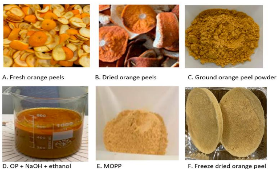
Figure 1. Pictorial presentation of various stages involved in preparing orange peels aerogels.
