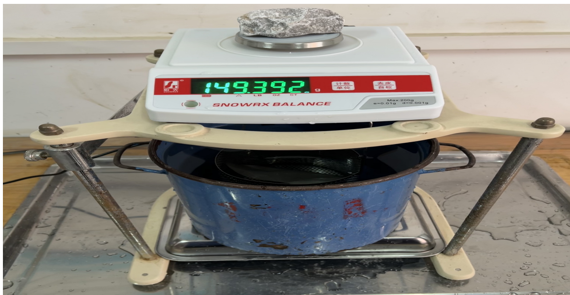
Figure 6. The image of the buoyancy balance used for the volume measurement.
