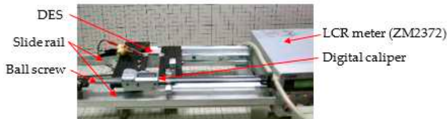
Figure 9. The test bench for the stretch DES.
