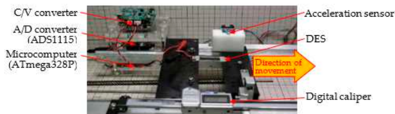
Figure 10. Measuring the response speed of a DES.
