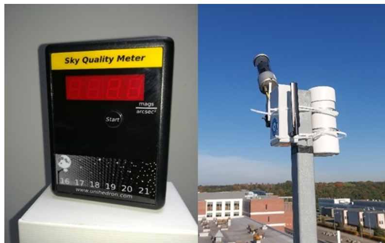
Figure 2. View of the hand-held SQM photometer (left, photo by Dominika Daab) and the automatic SQM photometer in the L version mounted on the observation deck of the Faculty of Earth Sciences and Spatial Management, Nicolaus Copernicus University in Toruń (right, photo by Mieczysław Kunz).
