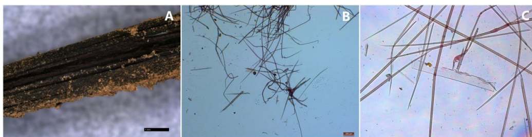
Figure 3. The microscopical pictures of the strip fiber (A: before chemical treatment, B and C: after chemical treatment).
