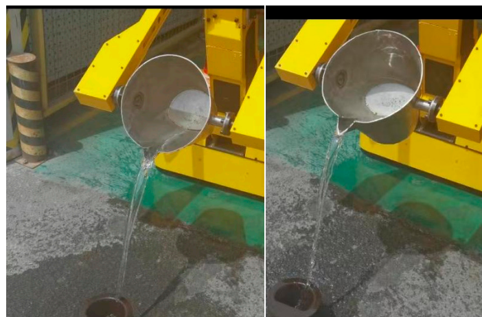
Figure 17. Pouring operation test.
