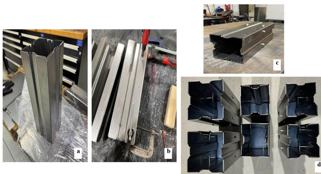
Figure 3. (a) and (b) Specimen before shear screw insertion (c) and (d) Specimen post shear screw insertion.
