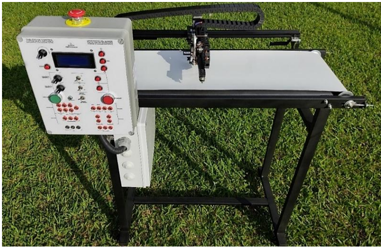
Figure 25. Building prototype of the flying cutting plant. Source: The authors.
