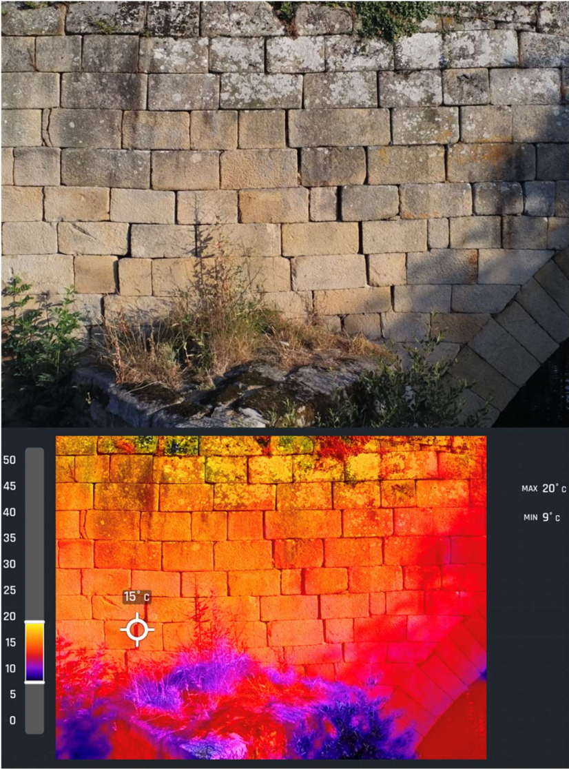
Figure 17. Photograph (upper figure) and thermogram (lower figure) of the central area of the spandrel wall, upstream of the bridge just above the starling (photograph by the author).
