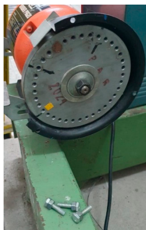
Figure 5. Balancing disc used in the static unbalance protocol (200 mm diameter, 10 mm thickness, 36 M12 holes every 10°). M12 screws of calibrated mass are inserted at controlled angular positions to induce or compensate unbalance, enabling reproducible generation of vibration signatures across a range of severities.
