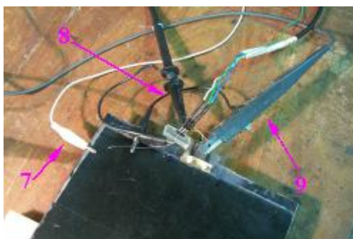
Figure 5. Measurement of the equivalent electrical impedance at 450 kHz with volt-amperometric method (Voltage probe TEKTRONIX Mod. P3010, current probe P6022 TEKTRONIX). The piezopolymer UGWIDT is bonded to the CFRP cross ply laminate.
