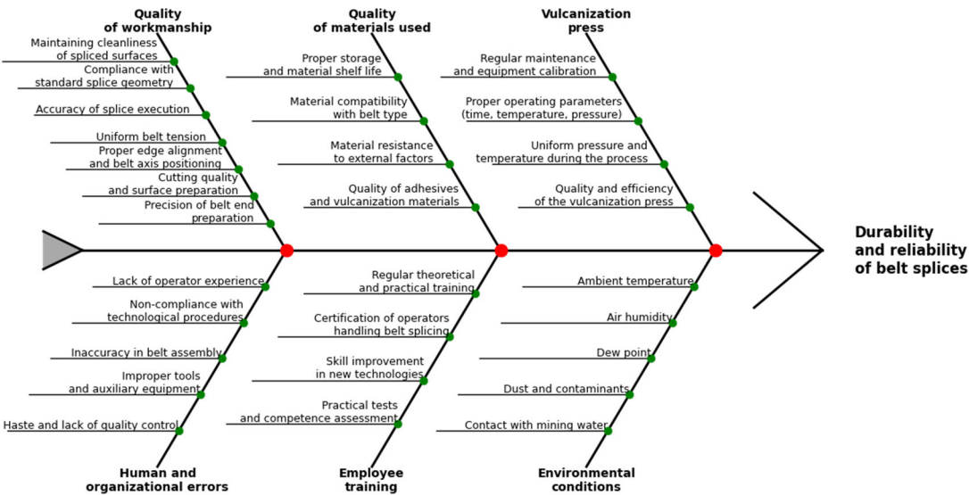
Figure 3. Ishikawa diagram showing factors affecting splice durability and reliability.
