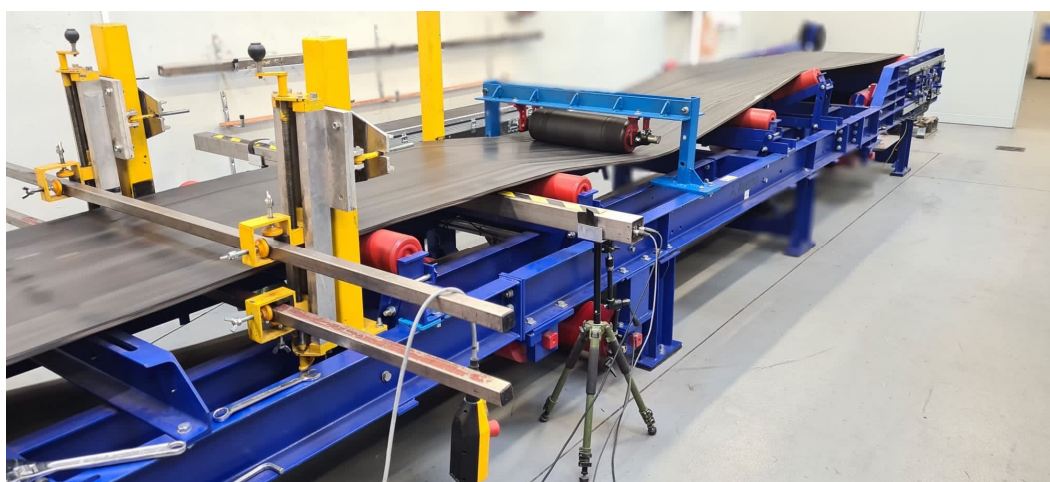
Figure 8. DiagBelt+ measurement system installed on the conveyor belt in the Belt Transport Laboratory during measurements.
