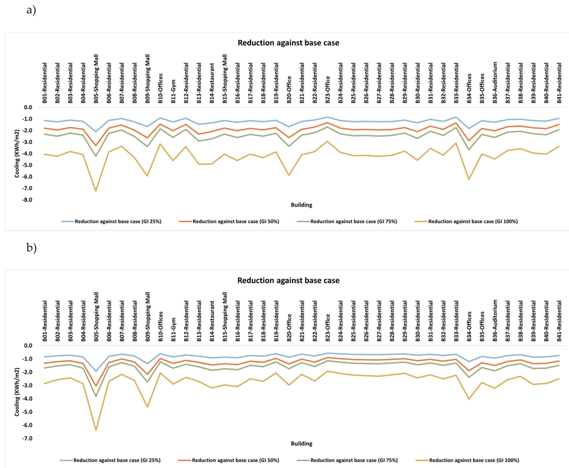
Figure 7. a) Reduction in cooling load against reference case (kWh/m 2 ) in all uninsulated buildings (commercial and residential) for base case and four heat mitigation scenarios (M1, M2, M3 and M4) in the summer month. b) Reduction in cooling load against reference case (kWh/m 2 ) in all insulated buildings (commercial and residential) for base case and four heat mitigation scenarios (M1, M2, M3 and M4) in the summer month.
