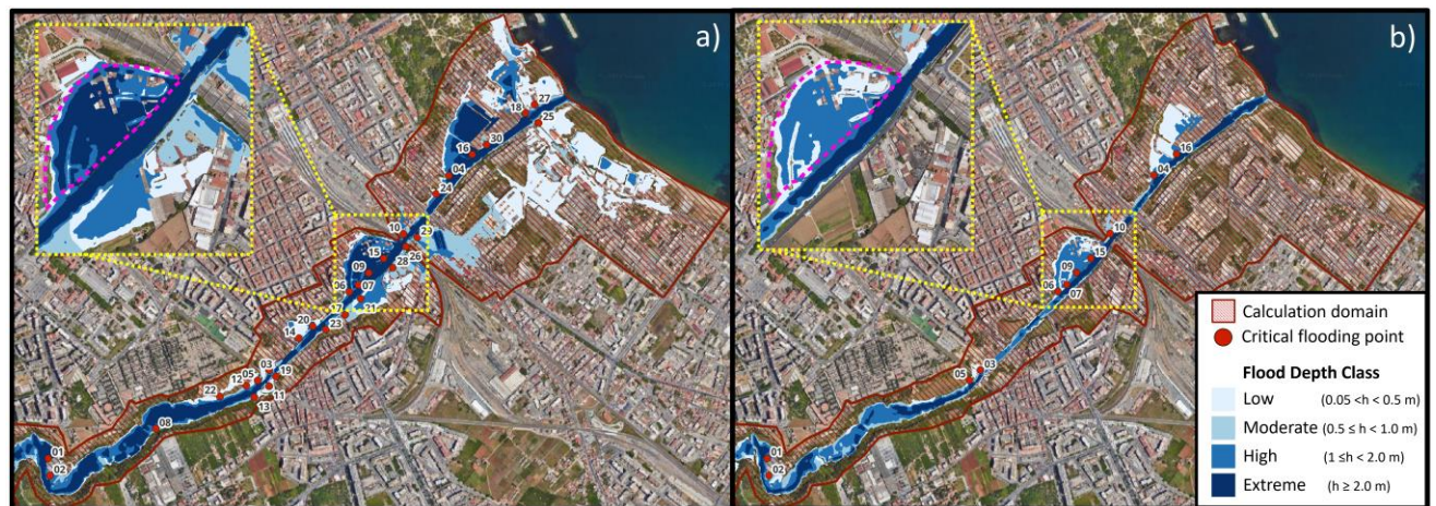
Figure 14. Flood Maps of the FESs Q0400HF (a) and Q0200HF (b), resulting from the application of the EWS based on the NMB 1 (bulletin of Nov. 2 nd , 2018) and NMB 2 (bulletin of Nov. 3 rd , 2018), respectively. A comparison of both maps with the actual flooded area (dashed magenta contour) in the district of Fondo Picone is reported in the insets.
