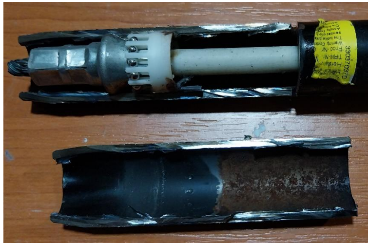
Figure 5. Example of cylinder deformed following the functioning of the anti-return pretensioning mechanism PBP.
