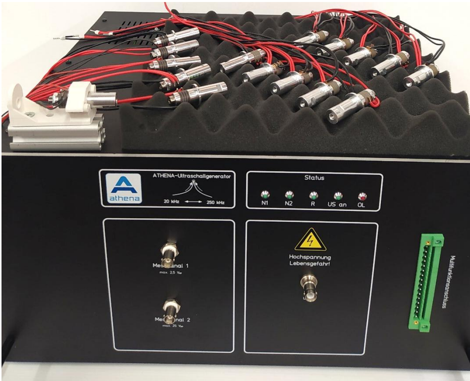
Figure 3. Series of assembled transducers with PZT and lead-free piezoelectric ceramics, plastics mounting bracket, and ATHENA ultrasound generator being used for resonance-controlled operation and measurements.
