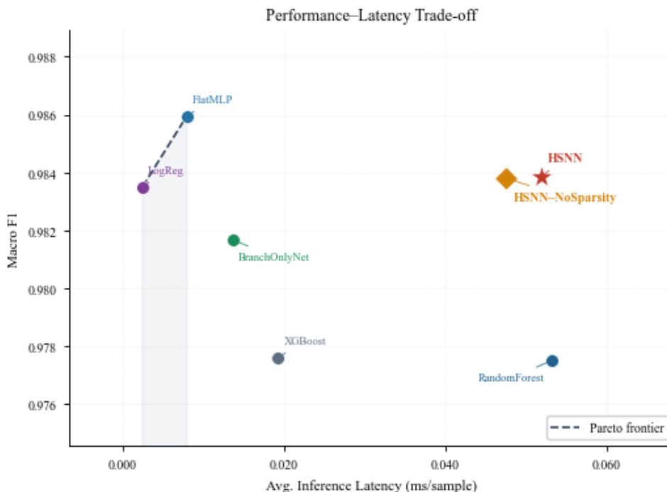
Figure 5. Performance–latency trade-off across models. HSNN strikes a good balance between detection performance and model size, keeping accuracy close to the top while using fewer parameters. However, it has a longer inference time than FlatMLP.
