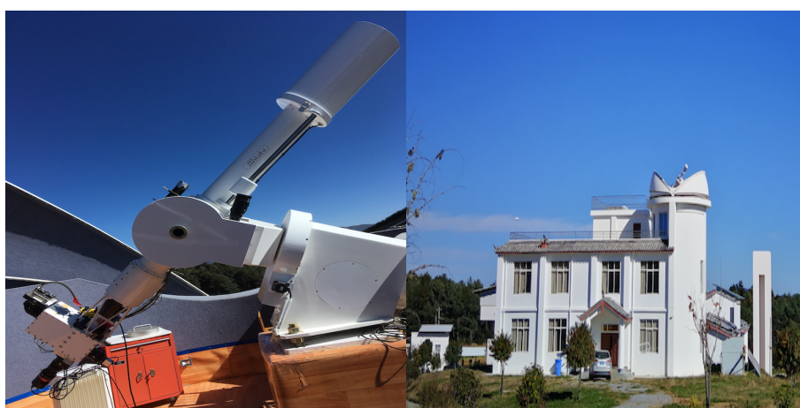
Figure 4. Light: YOGIS operates on the newly constructed platform, ensuring the regular coronal monitoring capability of the coronagraph. Right: This is the high-altitude coronagraph test base, dedicated to conducting ground-based coronagraph testing and experimental research; China's independently developed regular-operation coronagraph underwent its trials right here.
