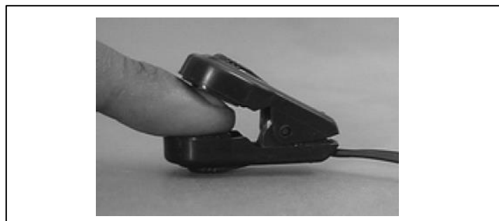
Figure 2. IR transmitter and receiver attached to the finger. Source: (Ibrahim & Buruncuk, 2005).
