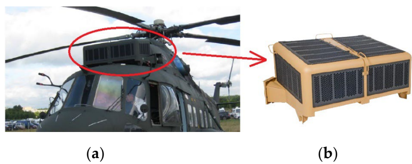
Figure 23. PURE air intake air filtration system for the multi-purpose Mi-17/Mi-8MT helicopter engine: (a) filter location, (b) view of the multicyclone constructed from VTS cyclones [72].
