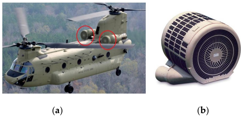
Figure 24. PURE air intake air filtration system for the multi-purpose engine of the CH-47 Chinook helicopter: (a) filter location, (b) view of the multicyclone constructed from VTS cyclones [73].
