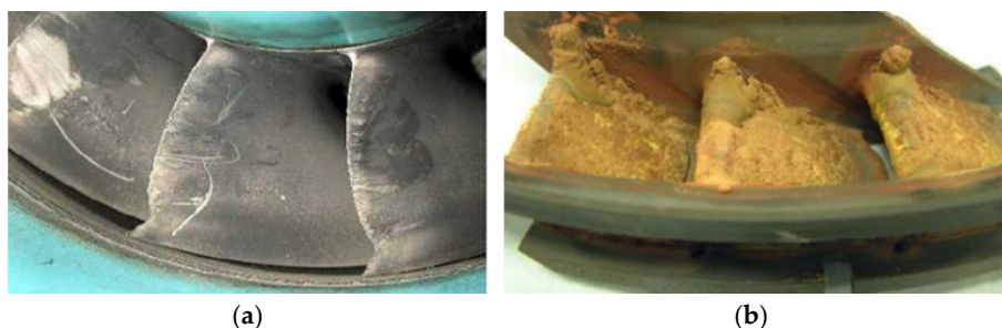
Figure 5. Impact of solid particles on turbine engine components: (a) erosion of the front and rear edges of compressor blades, (b) agglomeration of molten contaminants on turbine blades [11,32].
