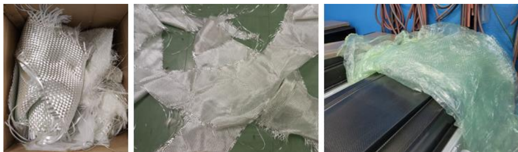
Figure 1. Typical waste from composite manufacturers: residuals of dry glass fiber fabrics, and used thermoplastic films.
