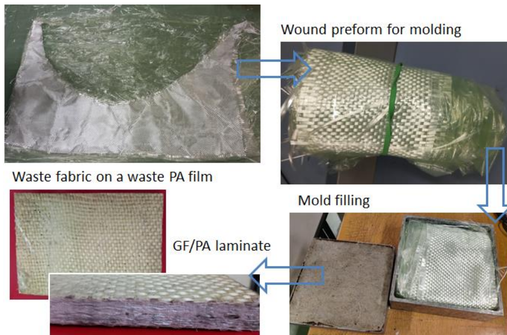
Figure 10. Fabrication of a 100% recycled GF/PA laminate with waste dry glass-fiber fabrics and waste PA films for vacuum bagging of composites.
