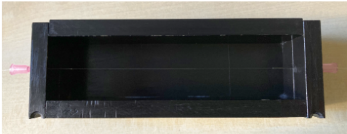
Figure 4. FOS placed in the mold before casting.
