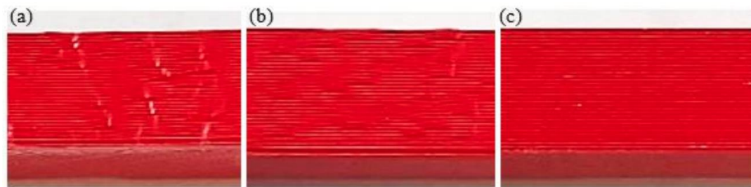
Figure 2. Side wall of specimens at different printing temperatures. (a) 180°C, (b) 190°C, (c) 220°C. [25].
