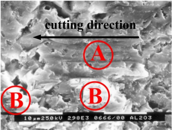
(a) Plastic deformation at position A and brittle fracture at position B
