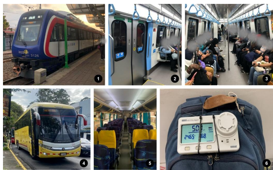
Figure 3. Pictures 1 to 3 present the exterior (1) and interior cabins (2 and 3) of the Diesel Multiple Unit (DMU) trains. Pictures 4 and 5 show the exterior and interior of the buses, respectively. Picture 6 displays the CO 2 measurement equipment and illustrates how the sensors were securely attached to the backpack.
