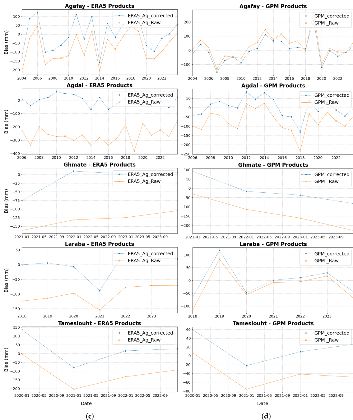
Figure 10. Graphical illustration of bias evolution of raw and corrected data of rainfall products (ERA5_Ag and GPM), blue dashed lines indicate corrected data, yellow lines indicate raw data, (a) ERA5_Ag monthly scale, (b) GPM monthly scale, (c) ERA5_Ag Annual scale, (b) GPM Annual scale.
