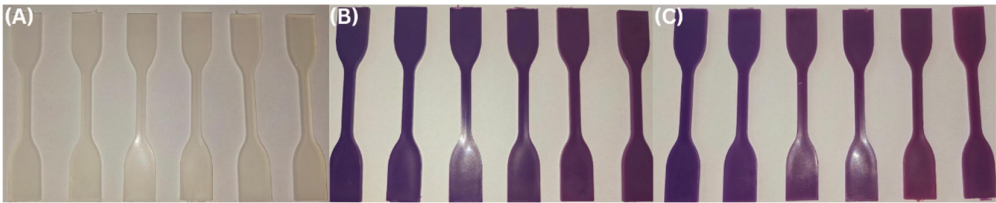
Figure 4. Injection-molded tensile test specimens. (A)—PP100/TP0 tensile test specimens after 0, 1, 2, 3, 4, and 5 recycling steps, (B)—PP98/TP2 tensile test specimens after 0, 1, 2, 3, 4, and 5 recycling steps, (C)—PP92/TP8 tensile test specimens after 0, 1, 2, 3, 4, and 5 recycling steps.
