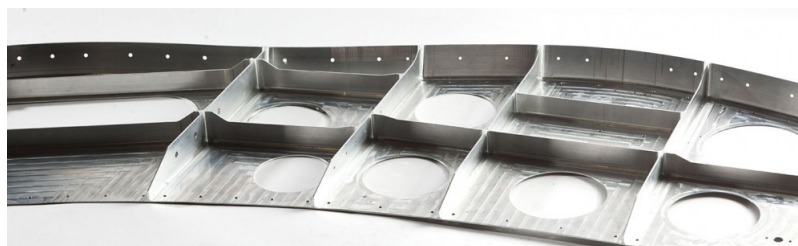
Figure 1. Example of pocketing in the aeronautical domain - Picture from OMNI - Aerospace inc [1]
