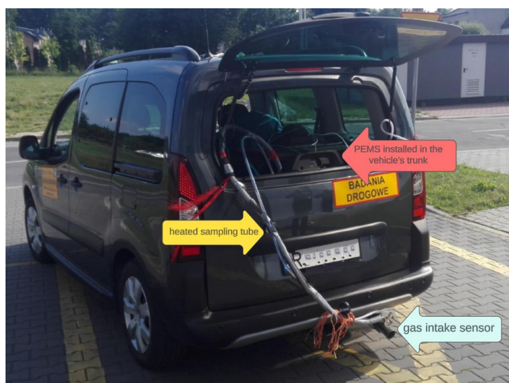
Figure 1. The vehicle selected for the study is equipped with a PEMS system.
