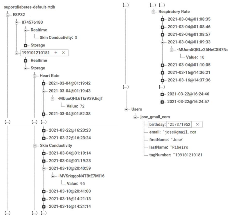
Figure 3. Firebase Data Storage Architecture and Exemplification. The database structure, in which data is stored inside "ESP32" node, while the "Users" node is used to store users' personal information, allowing data to be linked to the respective users through "tagNumber".
