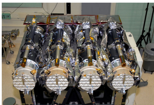
Figure 1. SDO project setup. All four telescopes adopt mirror coating.
