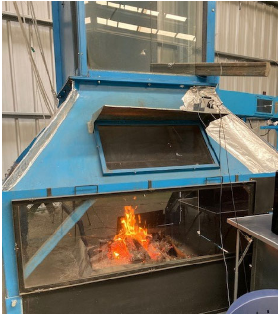
Figure 7. Vertical combustion tunnel, with wooden beam during the test.
