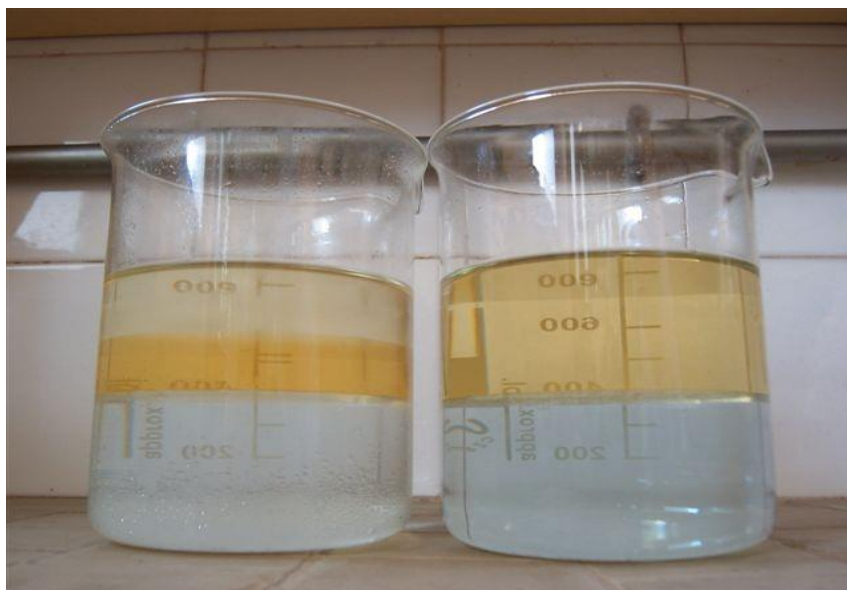
Figure 1. Undesirable third phase formation (left) in liquid-liquid extraction versus ordinary two phases systems (right). (Picture by F.J.Alguacil).
