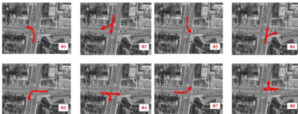
Figure 11. Different Phases of the Traffic Signal.
