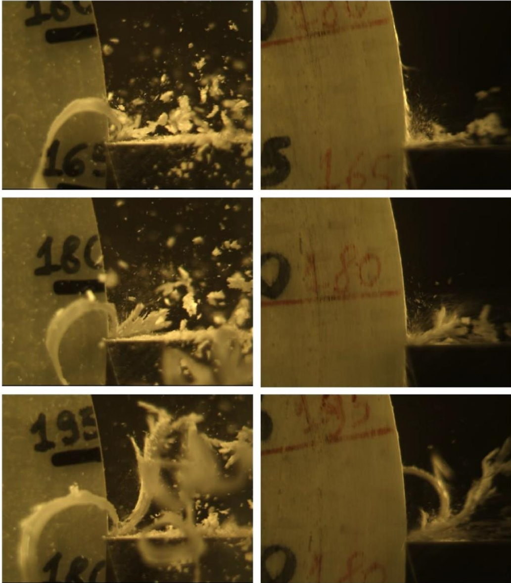
Figure 16. Chip morphology for circular specimens with (left) and without polycarbonate (right), around \theta = 180^\circ ( \gamma = 0^\circ , \alpha = 15^\circ , a_c = 0.20 mm, V_c = 50 m/min).
