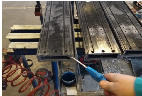
Figure 4. Dust removal after the machining phase.
