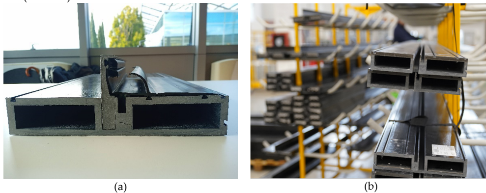
Figure 5. Basajaun bio-composite pultruded mullion profile specimens (a); Biobased profile preparation for façade prototypes after cutting and machining phase (b).
