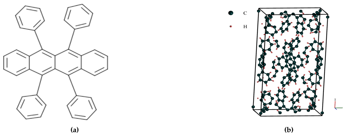
Figure 1. Molecular and Crystal Structure of Organic Semiconductor Rubrene
