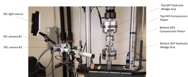
Figure 9. Compression Test Setup of Lattice Structures.
