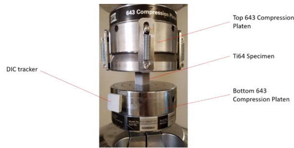
Figure 10. Close view of compression test fixture displaying the specimen and the.
