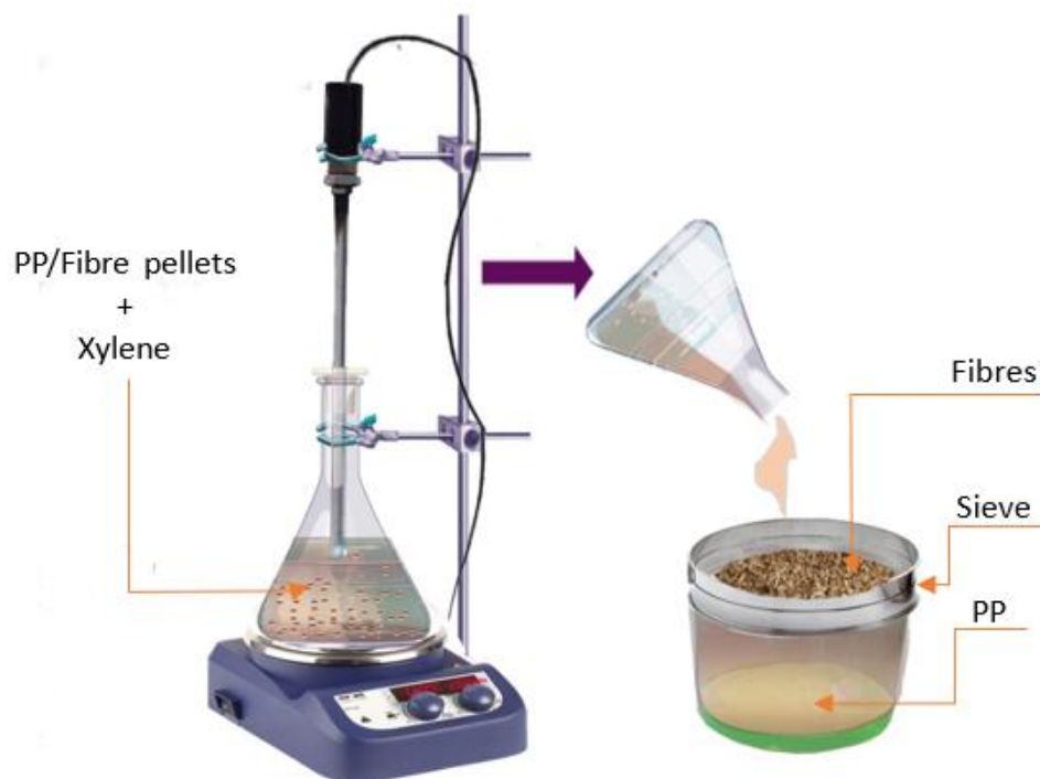
Figure 2. Fibre–matrix separation process.
